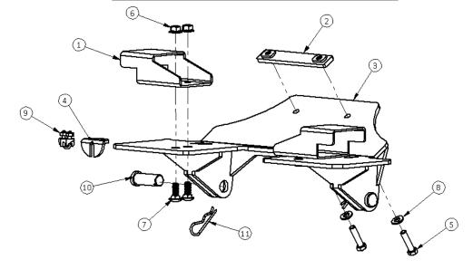
then fully tighten all of the hardware working in a crisscross pattern to keep the mount straight.
